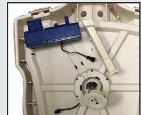
The Wire Cover and Clicker easily pop out by inserting a small flat-head screwdriver into the slots. For the Monitor, there is a screw next to the monitor lights in the front of the manikin to release it from the shoulder cavity (Phillips-head screwdriver needed).
